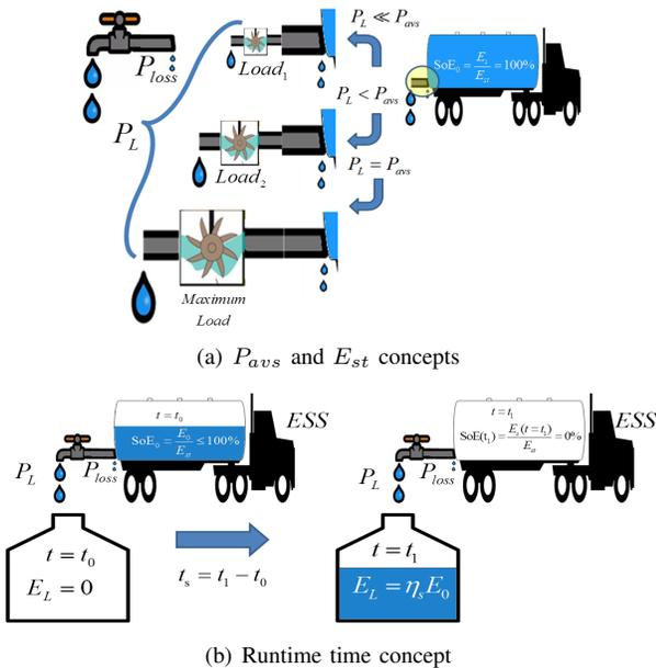
Fig. 2. Hydraulic analogy of a Loaded EPS.
