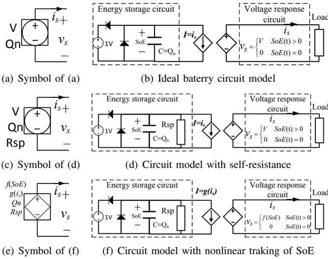
Fig. 3. DC voltage source with limited energy storage capacity
