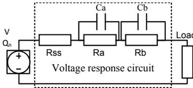
Fig. 4. Battery model proposed by [7] using the ideal battery model
