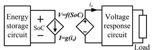
Fig. 1. Combined electrical-circuit based model.
