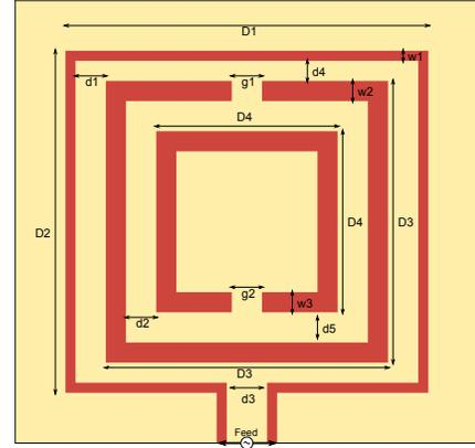
Fig. 3. Dimensions of the prototype on FR4 substrate in mm:  $D1 = 31.2$ ,  $D2 = 28.7$ ,  $D3 = 23.9$ ,  $D4 = 17$ ,  $d1 = 2.95$ ,  $d2 = 1.7$ ,  $d3 = 3$ ,  $d4 = 2.4$ ,  $d5 = 1.7$ ,  $g1 = g2 = 1$ ,  $w1 = 0.7$ ,  $w2 = w3 = 1.75$ .
