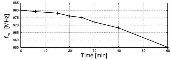
Fig. 6. Frequency at impedance matching condition of the FR4 prototype versus time due to variation of the relative humidity.
