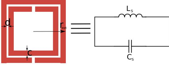
Fig. 2. Squared SRR structure and its simplified equivalent quasistatic model as an LC tank.
