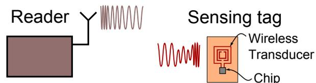
Fig. 1. Communication between reader and a wireless sensing tag. The tag includes the wireless transducer and a chip.
