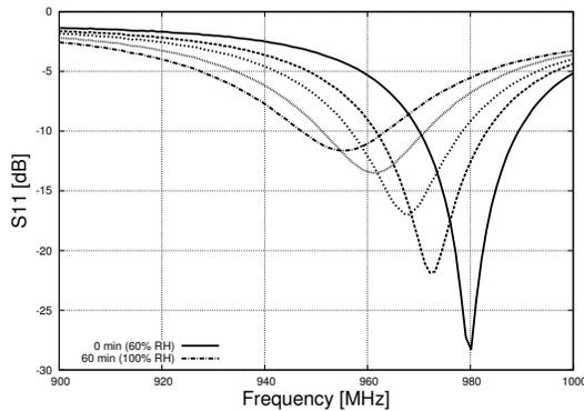
Fig. 5. Reflection coefficient variation of the FR4 prototype in response to relative humidity.
