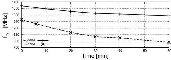
Fig. 8. Frequency at impedance matching condition of the paper prototype vs time (with and without PVA coating).
