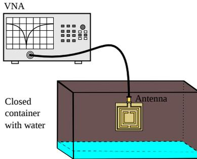
Fig. 4. Measurement setup for the humidity sensor.
