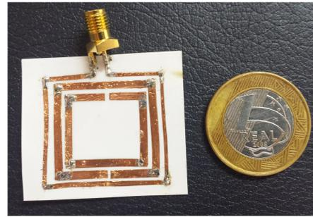
Fig. 7. Physical implementation of the wireless transducer on paper.
