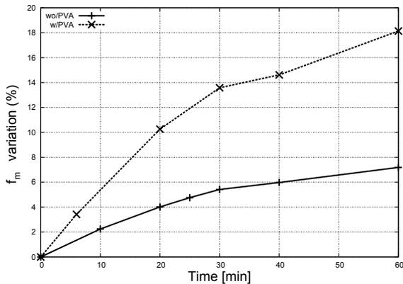
Fig. 9. Normalized percent variation of the frequency at impedance matching condition of the paper prototype vs time (with and without PVA coating).
