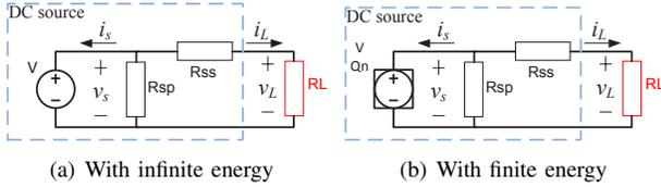
Fig. 3. Real DC voltage source models
