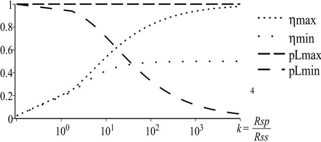
Fig. 8. Efficiency and load power boundaries vs k
