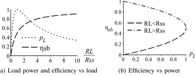
Fig. 6. PETO for a source w/o loss of self consumption
