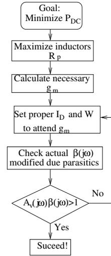
Fig. 3. Ultra-low-power oscillator design procedure flow chart
