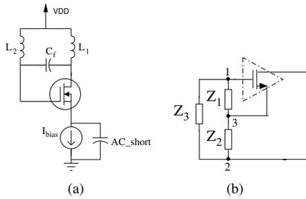
Fig. 1. Schematic diagram of designed oscillators: (a): Classical topology of Hartley oscillator; (b): Three-point oscillator equivalent circuit
