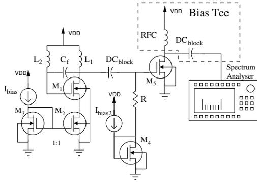
Fig. 4. Schematic of the ultra-low-power oscillator proposed
