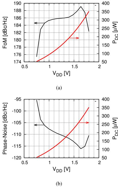
Fig. 5. Performance comparison: (a): FoM and  $P_{DC}$ ; (b): Phase-noise at 1 MHz of offset frequency and  $P_{DC}$
