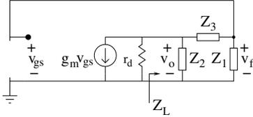
Fig. 2. Small-signal equivalent circuit
