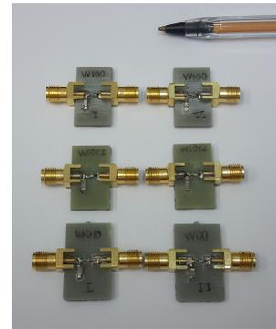
Figure 15: Impedance matching networks for 0%, 50% and 100% of water fractions.
